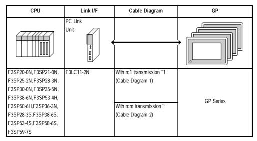
\* 1 The diagram below shows the system configuration recommended to allow n:m data transmission, using the host link protocol, between the Yokogawa Electric PLC [FA-M3] (or equipment supporting the same protocol - m units), and the GP (n units).
