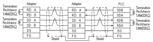
• When using Digital's Multi-link Cable, GP230-IS12-O
